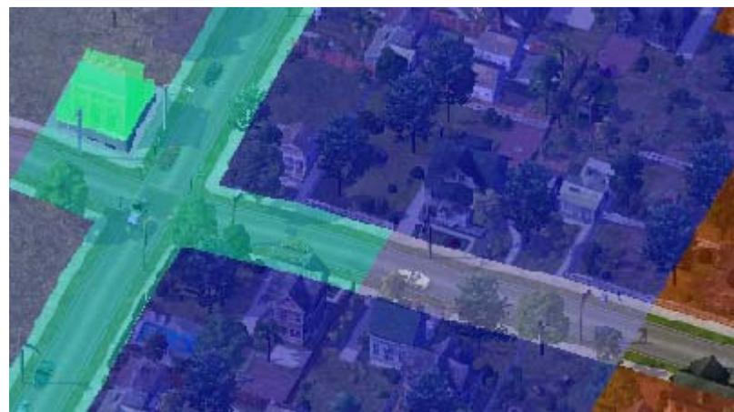
*Figure 2.* A screen shot of the Water data view depicting the water supply infrastructure. Blue indicates an area supplied with water, red indicates an area without water and green indicates a water supply facility or water main.
